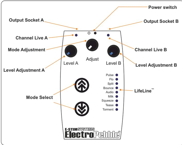
The ElectroPebble® has a number of user controls. Each control allows the user to adjust a particular aspect of the output.
